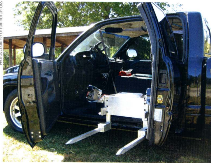
Standard installations of the vehicle-entry system are available for most full-size, extended-cab, two-wheel-drive pickup trucks offering "suicide" side doors.
